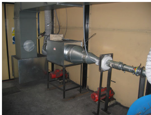
Fig. 4 Pilot plant adsorber for balancing of VOC concentrations in exhaust gas from the paint shop
